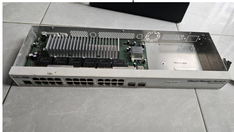
Fig. 5. Internal view of the MikroTik CRS326 switch after the incident. Although no visible burn marks are present, the device failed to operate, indicating internal damage caused by lightning-induced overvoltage.
