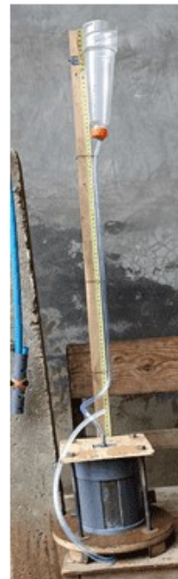
Figure 1. Falling Head Permeability Test Equipment
