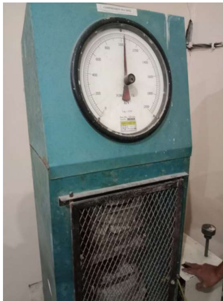
Figure 4. Paving Block Compressive Strength Test Process
