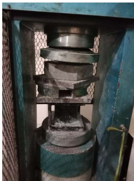
Figure 3. Test Compressive Strenght
