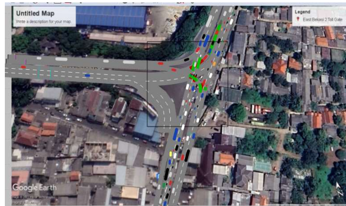
Figure 5. Simulation of the existing Exit Ramp and Simpang East Bekasi 2 Source: Vissim Analysis Results, 2025
