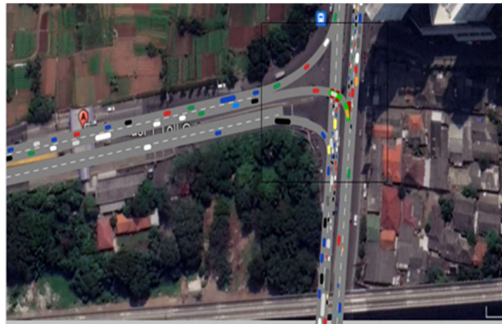
Figure 4. Simulation of the existing Exit Ramp and Simpang East Bekasi 1 Source: Vissim Analysis Results, 2025
