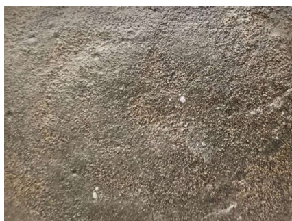
Figure 1. Saturated sand condition (moisture content: 28%).
