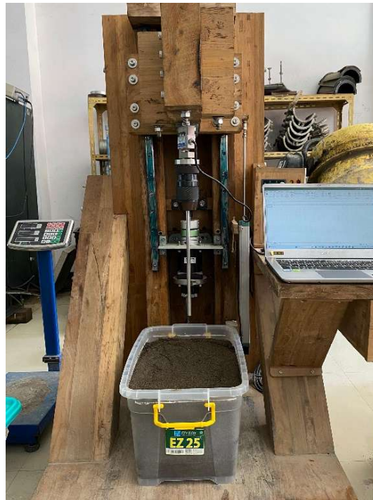
Figure 4. Automatic axial loading apparatus with real-time data (AIC Innovation) [29].
