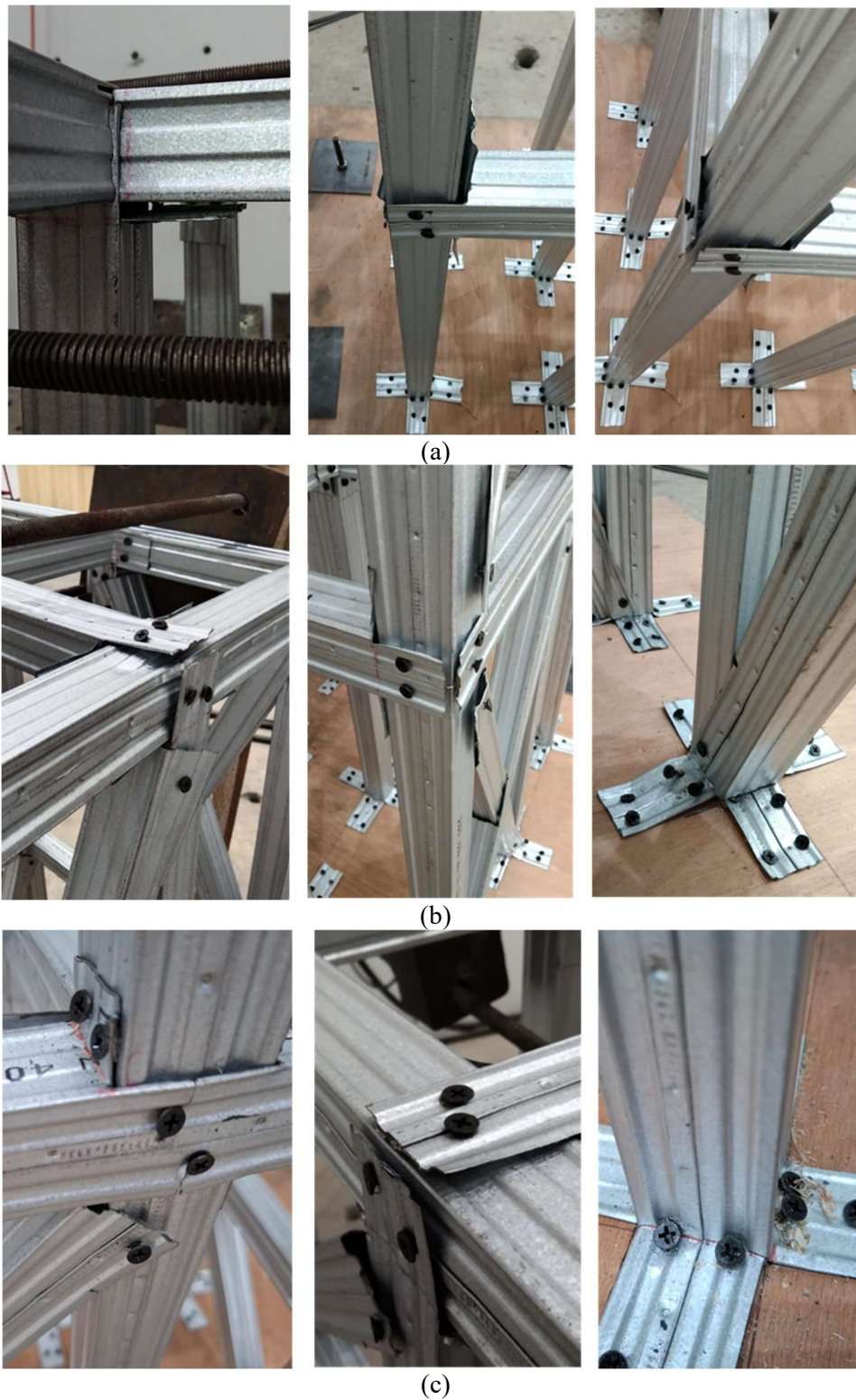
Figure 12. Connection Failure in No-Brace (a), Connection Failure in X-Brace (b), and Connection Failure in Z-Brace ©
