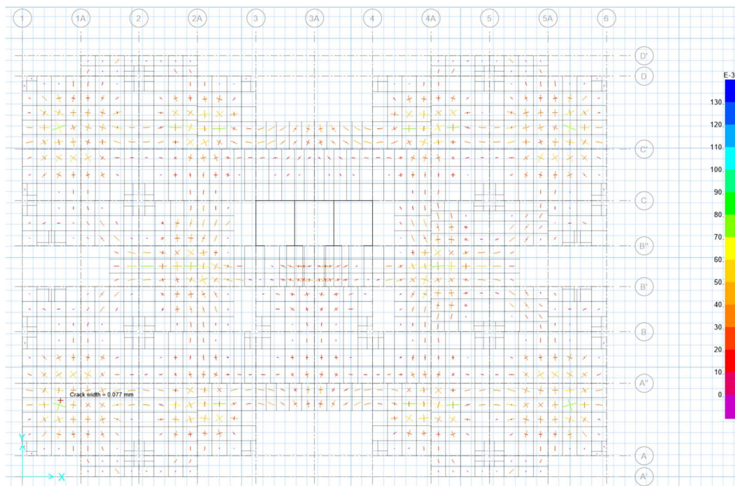
Figure 8. Long-term crack values in SAFE.
