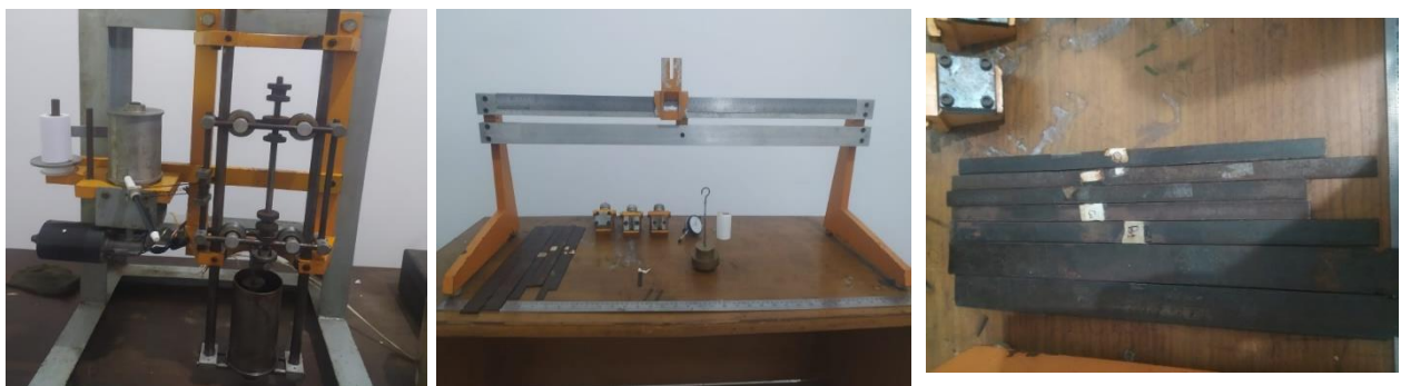
Gambar 1. a. Simple Vibration Apparatus , b. Beam Deflection Apparatus , c. Spesimen uji
