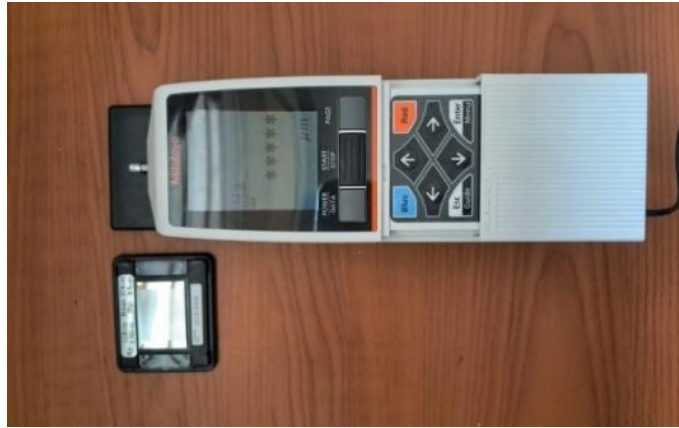
Gambar 4. Mitutoyo Surface Roughness Tester SJ-210
