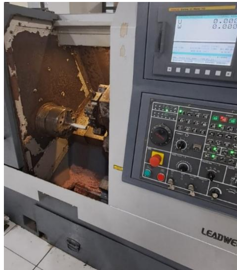
Gambar 2. LEADWELL CNC Lathe Fanuc Oi Tc
