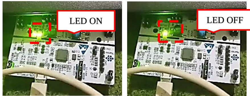
Figure 3. Testing STM32 Led on and Led off Source: Personal Documents
