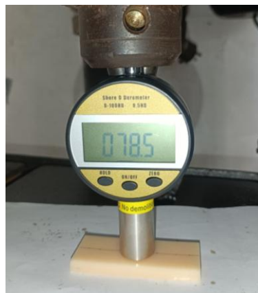
Figure 6. Specimen Hardness Measurement Using Shore D Durometer
